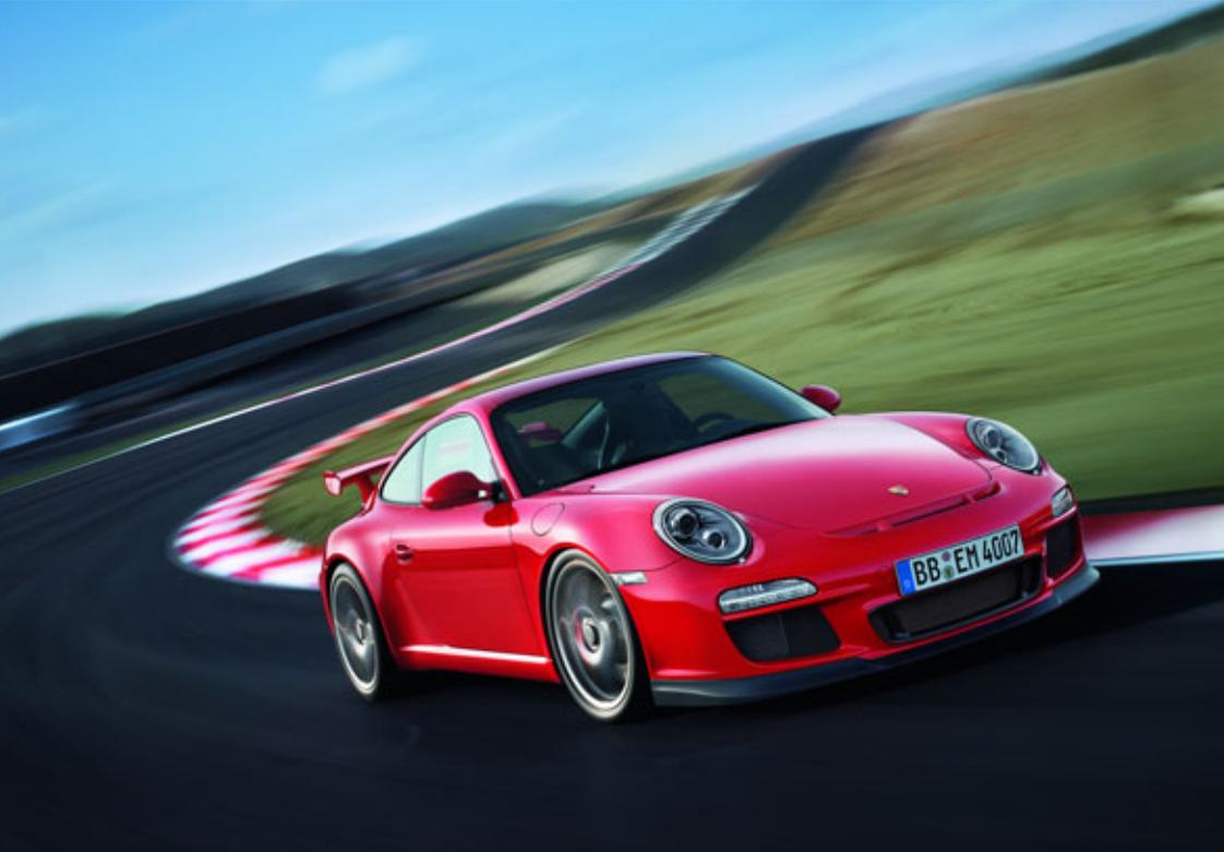
The wheel dimensions are 8.5J x 19 with 235/35 ZR 19 tyres (front) and 12J x 19 with 305/30 ZR 19 tyres (rear). Road-legal sport tyres provide the necessary grip, although the lower tread profile presents a greater risk of aquaplaning on wet roads.
