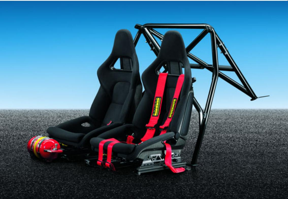
It consists of a roll cage that is bolted to the body behind the front seats, a six-point racing harness in red for the driver's side, a fire extinguisher with mounting bracket and preparation for a battery master switch. The Clubsport
